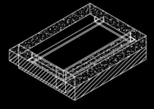
Load on the frame to be applied only after grouting is completed
