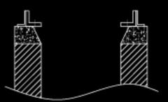
Wrong installation of frame as frame is not completely supported
